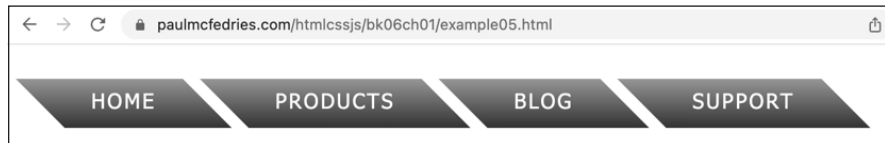
FIGURE BC1-5: The li::before pseudo-element is a square skewed into a parallelogram shape.
