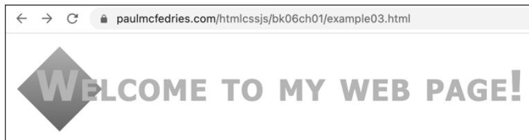
FIGURE BC1-3: The h1::before pseudo-element is a rotated square that appears behind the h1 text.
