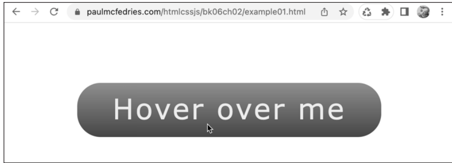
FIGURE BC2-2: The button scaled to twice its default size at the end of the transition.
