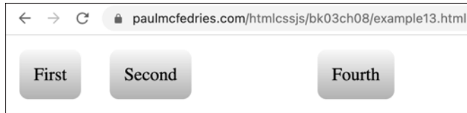
FIGURE BC4-11: The third div is invisible, but its box still takes up room in the layout.
